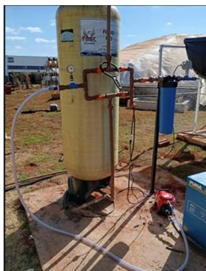
Figure 1. Biogas filter installed at test environment.
