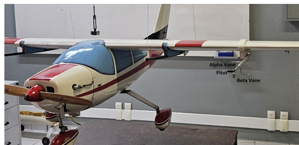
Figure 2. Anemometric sensors for measuring angles of attack and sideslip installed on the Cessna 177B subscale model.
