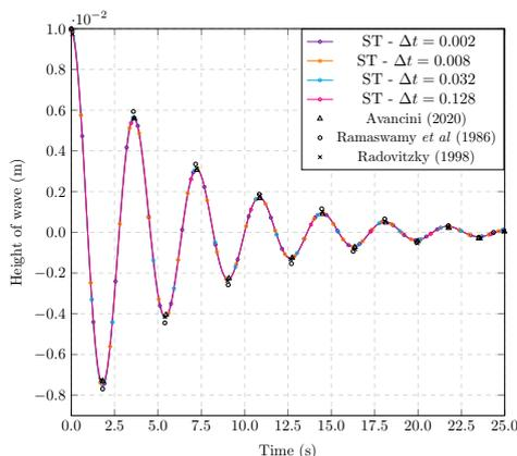
Figure 2. Wave height on the right wall - Analysis considering four different time steps and comparison with literature results.
