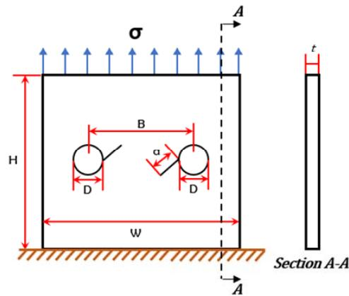
Figure 5. Aluminum alloy properties and plate with double hole edge crack (geometry and boundary conditions)
