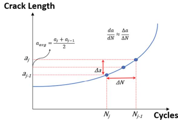
Figure 1. Crack length versus number of cycles
