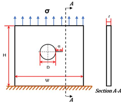
Figure 2. Aluminum alloy properties and plate with hole edge crack (geometry and boundary conditions)
