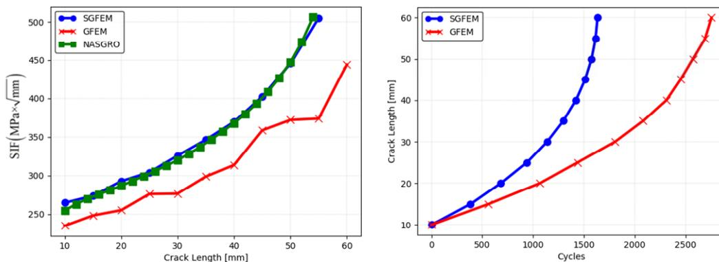
Figure 4. SIF results comparison (left) and number of cycles versus crack length (right) for plate with hole edge crack.
