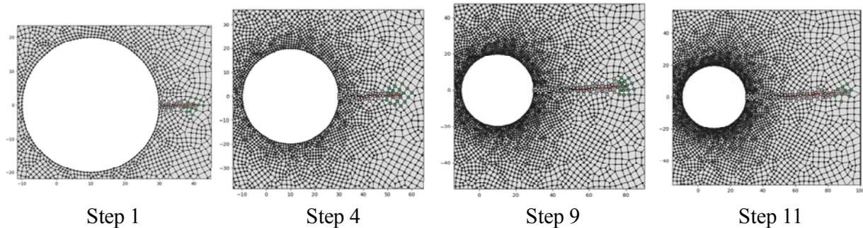
Figure 3. Some crack propagation steps for plate with hole edge crack. Green nodes are enriched by singular functions, white nodes are enriched by Heaviside functions (constant and linear) and also linear polynomial functions.
