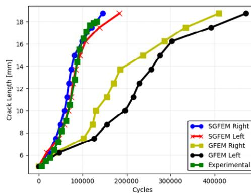
Figure 7. Number of cycles versus crack length (right) for plate with double hole edge crack
