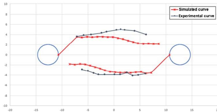
Figure 6. Crack path comparison between the simulation and experimental data for plate with double hole edge crack
