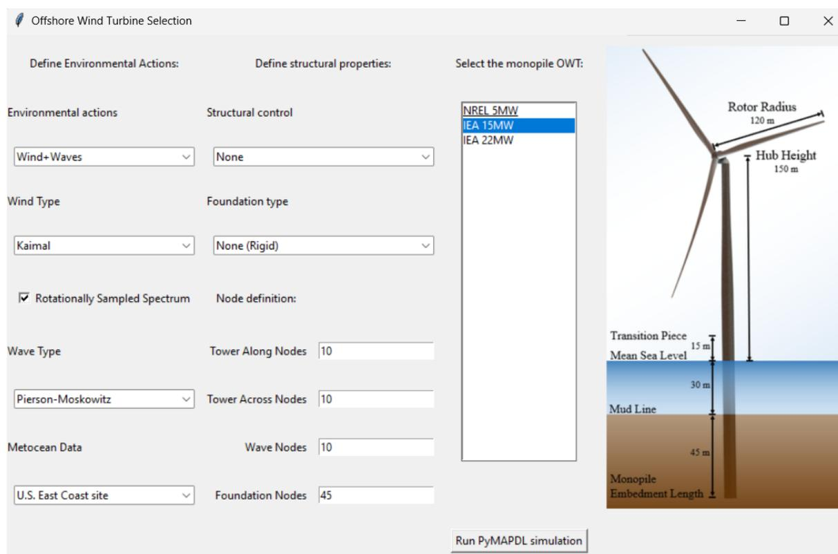
Figure 1. Graphical User Interface (GUI) for selecting and defining simulation parameters for OWTs.
