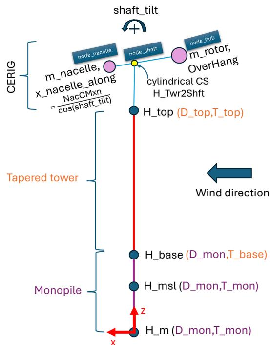
Figure 2. Input data for tower geometry.
