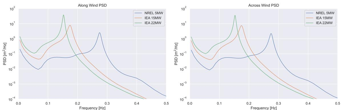
Figure 3. Power Spectral Density (PSD) responses of the NREL 5-MW, IEA 15-MW, and IEA 22-MW models. The left subplot shows the along-wind PSD response, while the right subplot depicts the across-wind PSD response.
