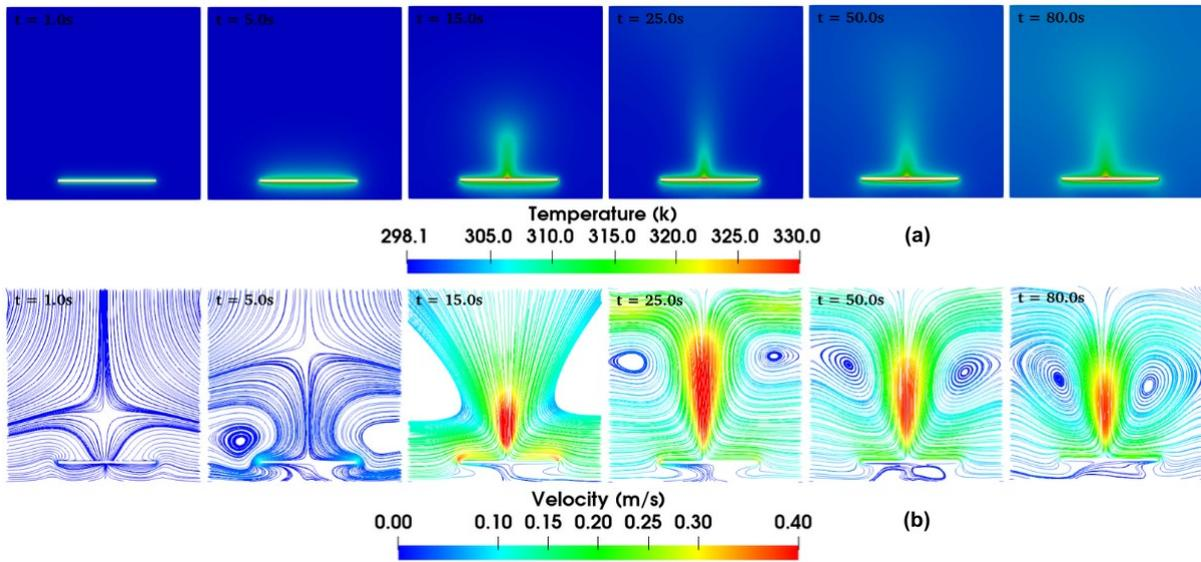
Figure 2. (a) Variation of the temperature field over time for the horizontal plate case. (b) Variation of the velocity field and air flow lines over time.
