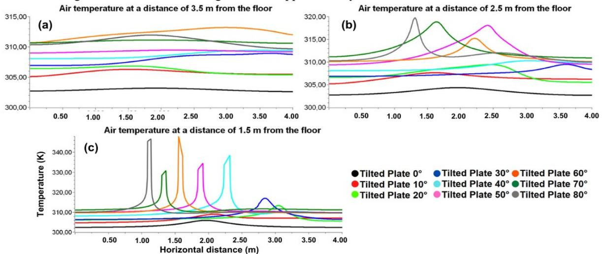
Figure 4. Comparison of fluid temperature values for different inclinations at vertical distances of 3.5 m (a), 2.5 m (b), and 1.5 m (c) from the ground.
