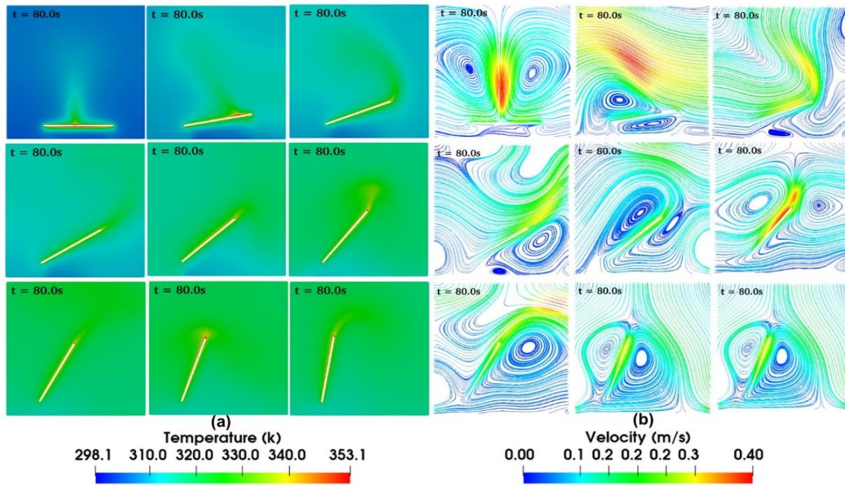
Figure 3. (a) Comparison of the temperature field for the different slopes. (b) Comparison of air flow lines for different inclinations.
