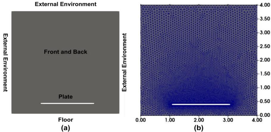
Figure 1. (a) Geometric model of the computational domain. (b) Pseudo-3D finite volume mesh.
