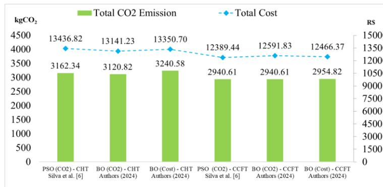
Figure 3. Comparative analyses of the solutions to the total CO<sub>2</sub> emission
