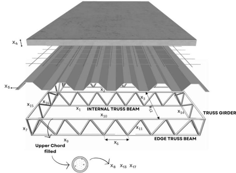
Figure 1. Design variables of the composite tubular-floor trusses
