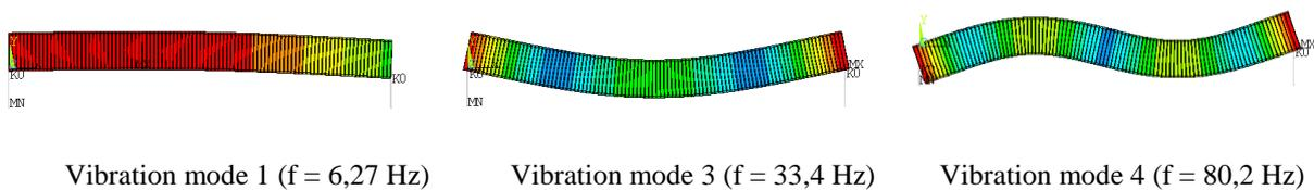
Figure 3. Vibration modes of the target model.
