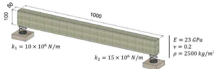
Figure 1. Schematic representation of the structure, dimensions in centimeters
