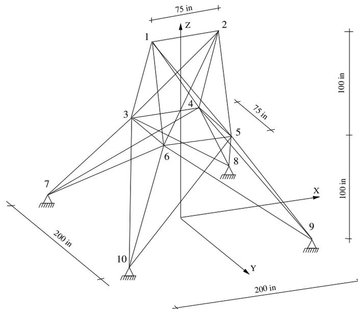
Figure 1. 25-bar truss.
