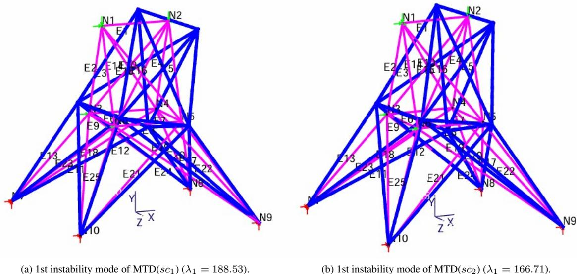
Figure 3. First instability mode of the MTD solutions. The original configuration of the 25-bar truss is represented in pink, and the deformed shape is colored in blue.
