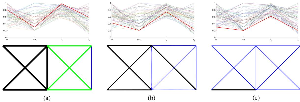
Figure 4. Extracted non-dominated solutions from MCDM for the 10-bar truss.
