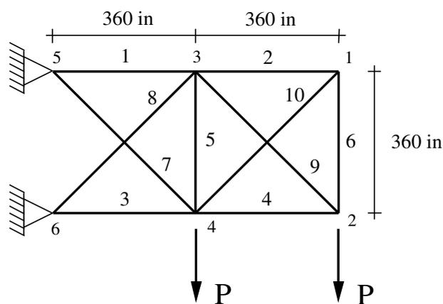
Figure 1. The 10-bar truss.
