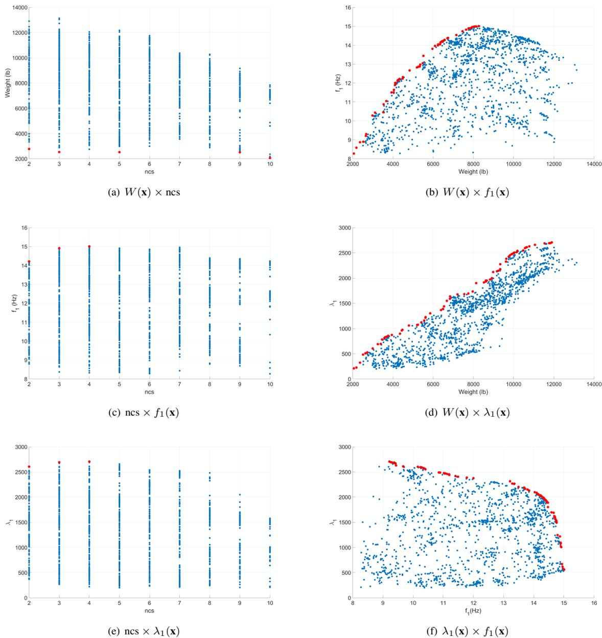
Figure 3. Non-dominated solutions for the 10-bar truss.
