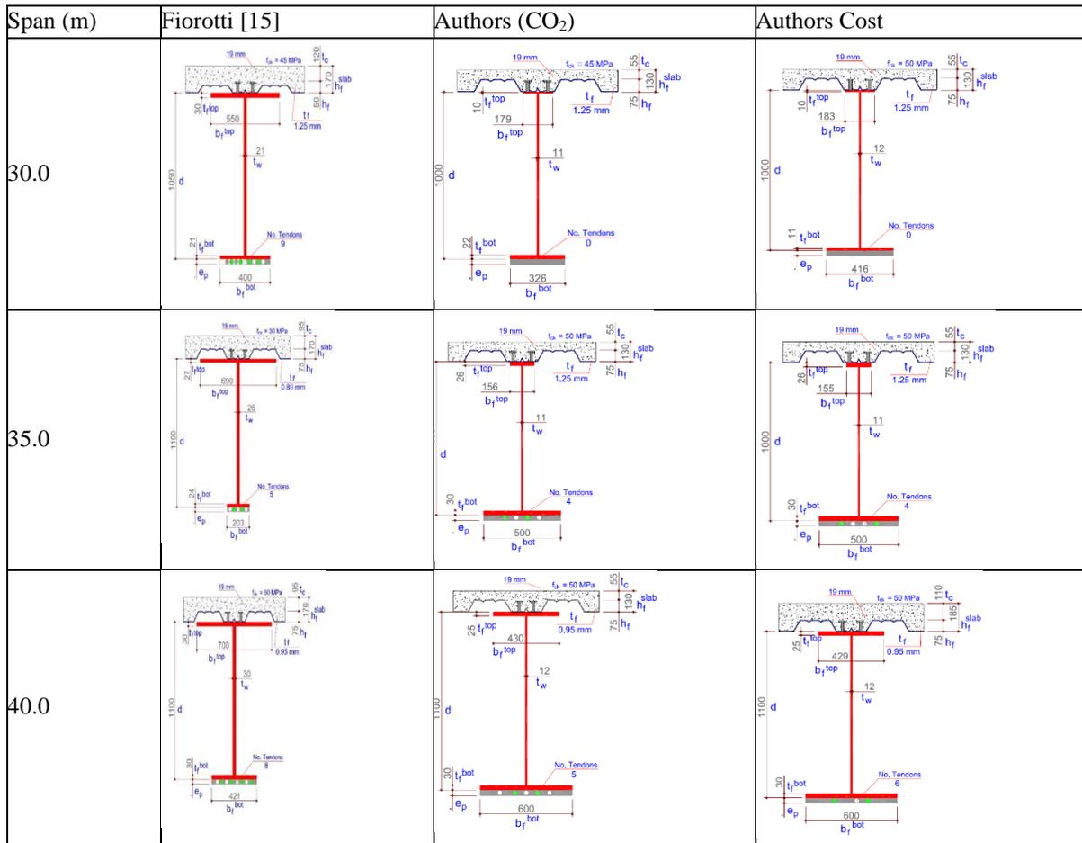
Figure 5 – Profiles found by the algorithm for each span.
