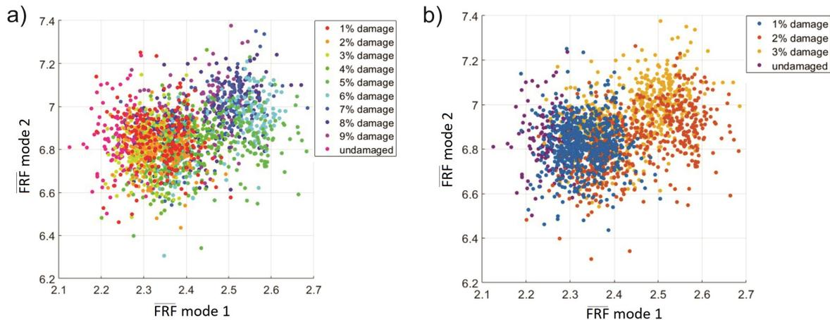
Figure 4. Damaged and undamaged samples generated from numerical simulations, a) dataset considering 9 damage levels and b) dataset considering 3 damage levels.
