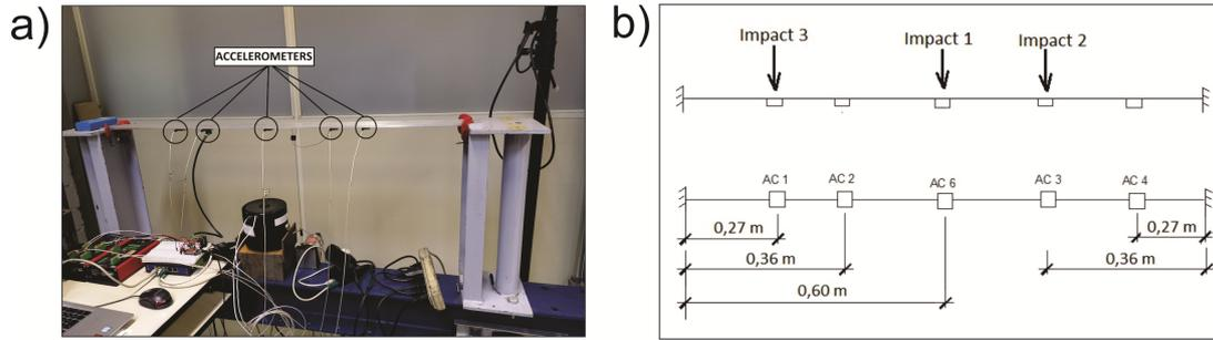
Figure 1. Experimental setup for dynamic testing (Ruiz et al. [10]). a) test structure, b) accelerometers' positions and excitation points.
