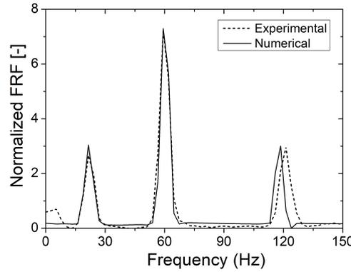
Figure 3. Comparison between numerical and experimental FRFs.
