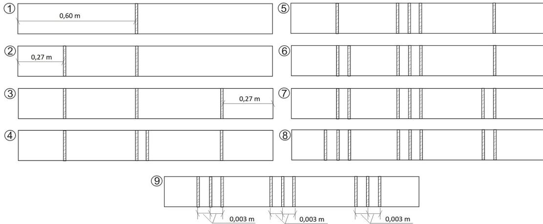
Figure 2. The nine damage scenarios induced on the beam.
