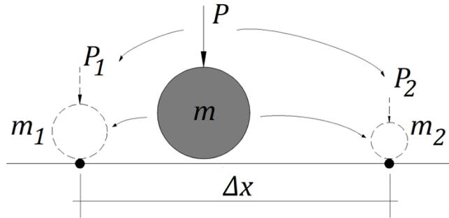
Figure 4. Distribution of masses and loads between nodes
