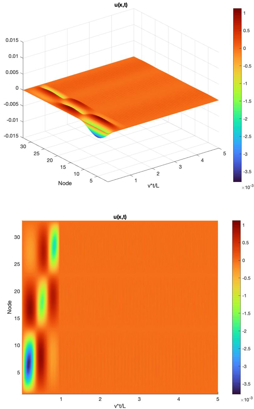
Figure 6. Transversal response of the undamped structure under mobile load, for displacement speed of 10.00m/s
