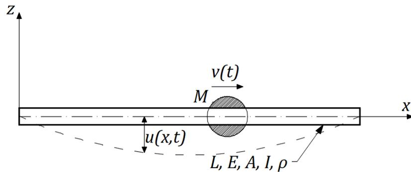
Figure 2. Simply supported beam subjected to a moving mass system.
