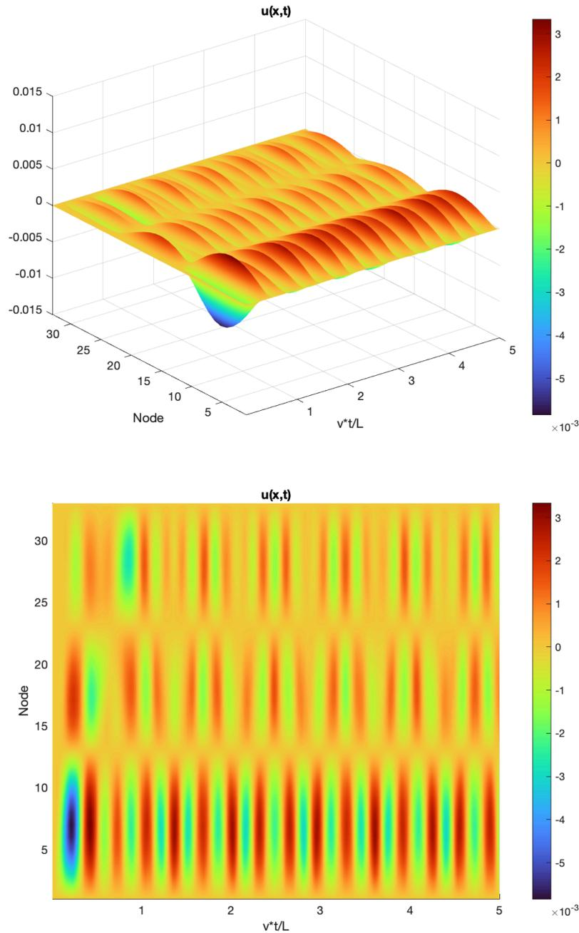
Figure 7. Transversal response of the undamped structure under mobile load, for displacement speed of 90.00m/s
