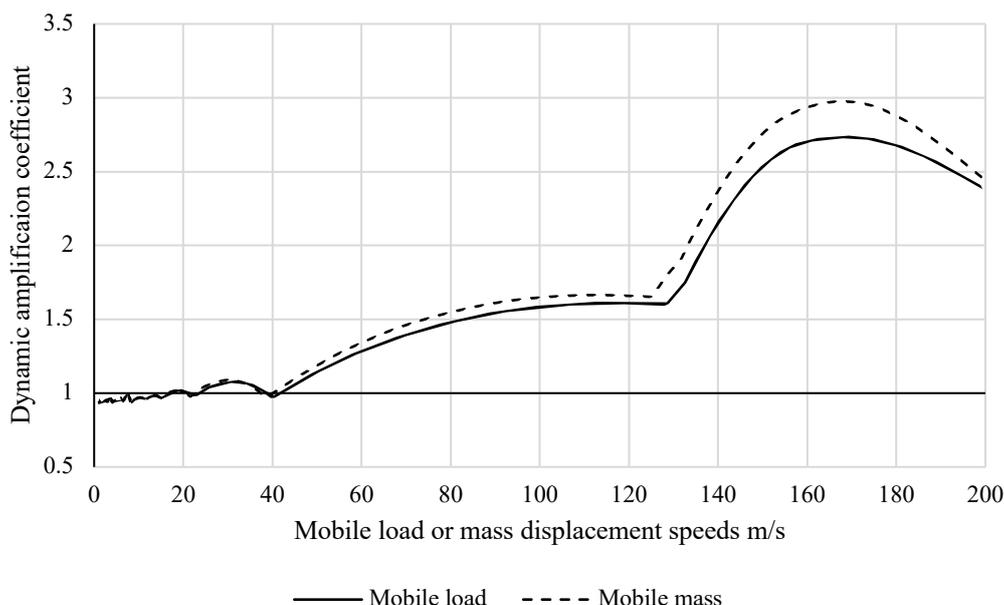
Figure 8. Relation between the displacement speed of the mobile load and mobile mass and the dynamic amplification coefficient for three span continuous beam
