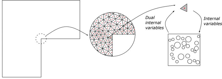
Figure 2. Representation of the homogenized macroscale and the heterogeneous microscale models. Observe that a heterogeneous microscale model is associated for each macroscale integration point. The FE<sup>2</sup> process occurs by transferring internal variables from macro to microscale and dual internal variables from micro to macroscale.
