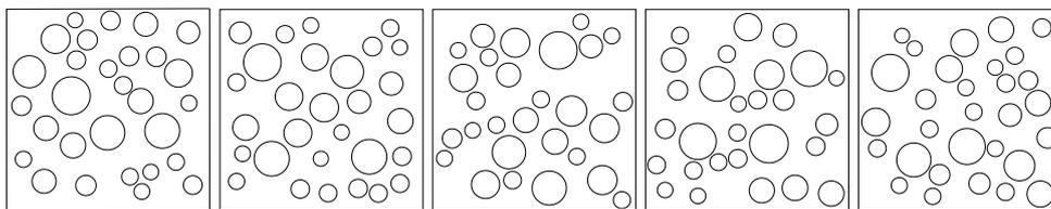
Figure 4. RVEs with random particle distributions for a volume fraction of 30%.
