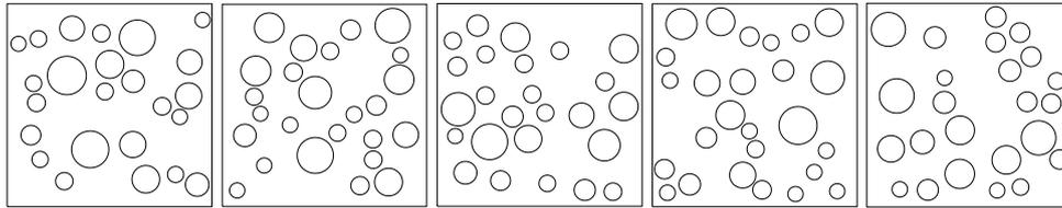
Figure 3. RVEs with random particle distributions for a volume fraction of 25%.
