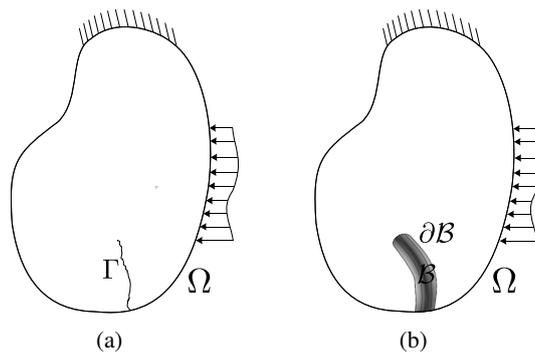
Figure 1. Comparison between (a) Griffith crack and (b) Phase-Field diffuse crack
