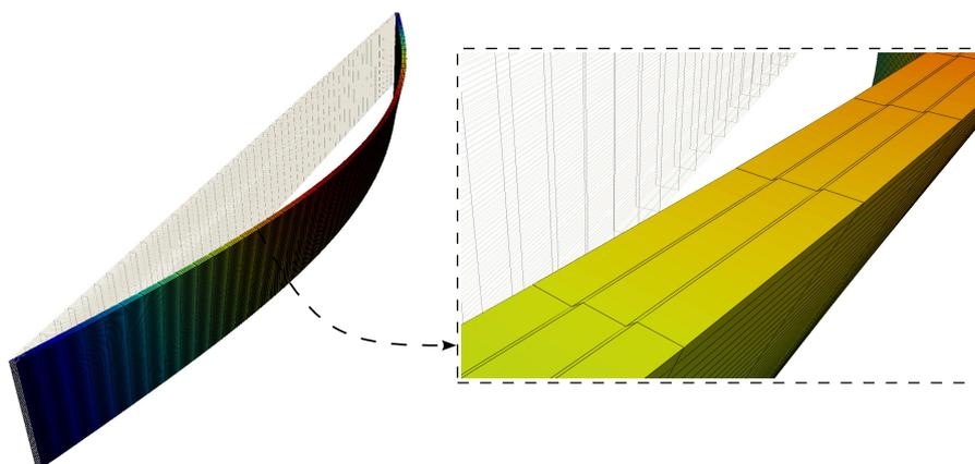
Figure 5. Lateral torsional buckling mode for CS3.
