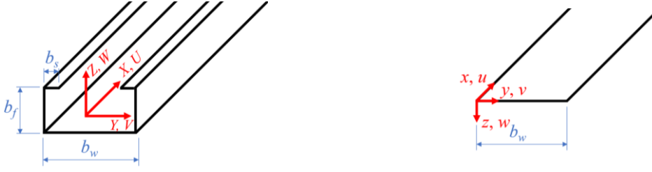
Figure 1. Coordinate systems adopted: (a) global (X-Y-Z), and (b) local (x-y-z). Adapted from [13, 14].
