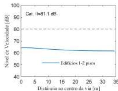
Figure 8. Prediction of vibration levels in terms of maximum Running RMS values inside a typical building.
