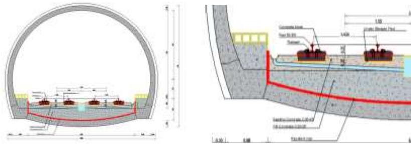
Figure 3. Track cross-section.
