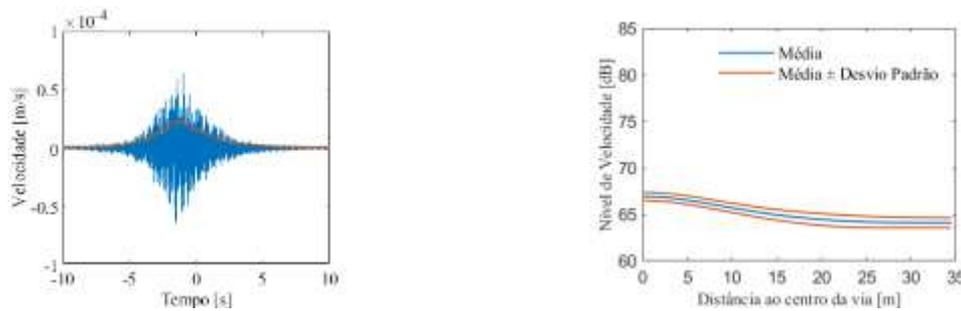
Figure 7. Vibration velocity record evaluated at the ground surface for the passage of the EuroTram vehicle.
