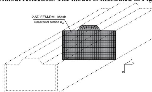
Figure 1 . Infinite and invariant structure in one direction – 2.5D FEM-PML approach.
