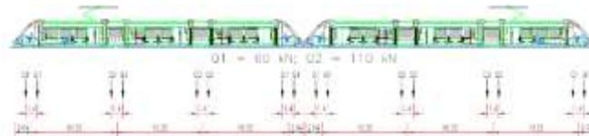
Figure 4. Geometrical configuration and axle loads of the vehicle EuroTram.
