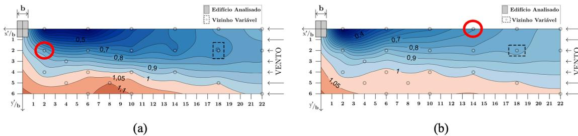
Figure 4 – Highlight for Interference Factor of (a) oblique and (b) aligned neighbors. Source: Lavôr [4]
