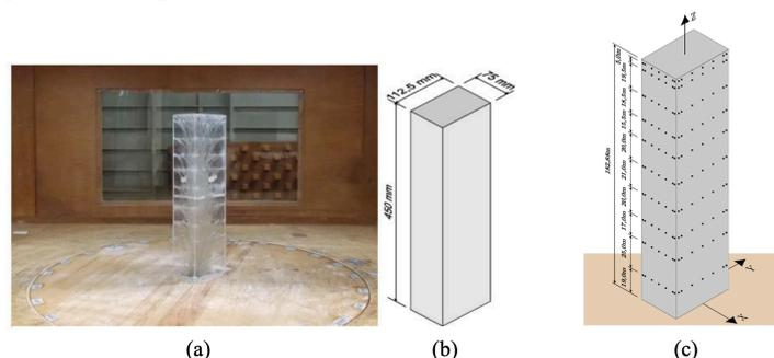
Figure 1. (a) CAARC instrumented with pressure taps; (b) model dimensions; and (c) Full-scale CAARC standard tall building and positions of the pressure taps. Source: Lavôr [4]
