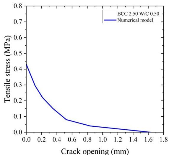
Figure 10. Tensile stress versus crack opening curve BCC 2.50 W/C 0.50
