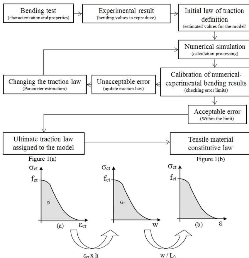
Figure 1. Process of drawing up a tensile law by inverse analysis
