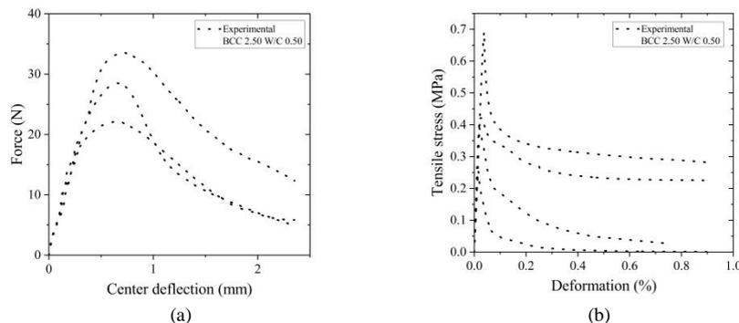
Figure 4. Experimental curve ranges of BCC 2.50 W/C 0.50 bamboo bioconcrete: (a) three-point bending; (b) direct tension test. Adapted from Andreola [2]
