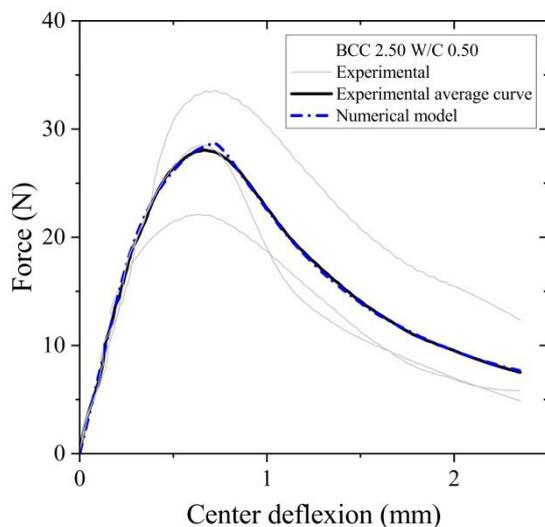
Figure 9. Force versus displacement curves BCC 2.50 W/C 0.50
