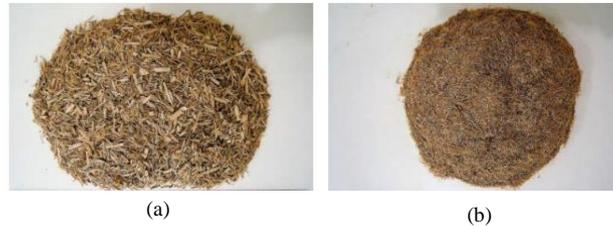
Figure 3. Bamboo particles used in the composition of bioconcrete: (a) particles retained on the #1.18 mm sieve; (b) fine particles passing the #1.18 mm sieve. Adapted from Andreola [2]
