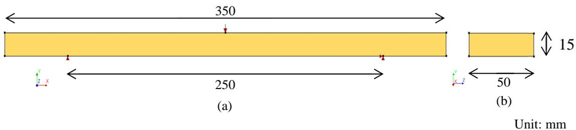
Figure 5. Numerical model: (a) geometry details; (b) cross section
