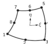
Figure 6. Finite element type CQ16M [5]
