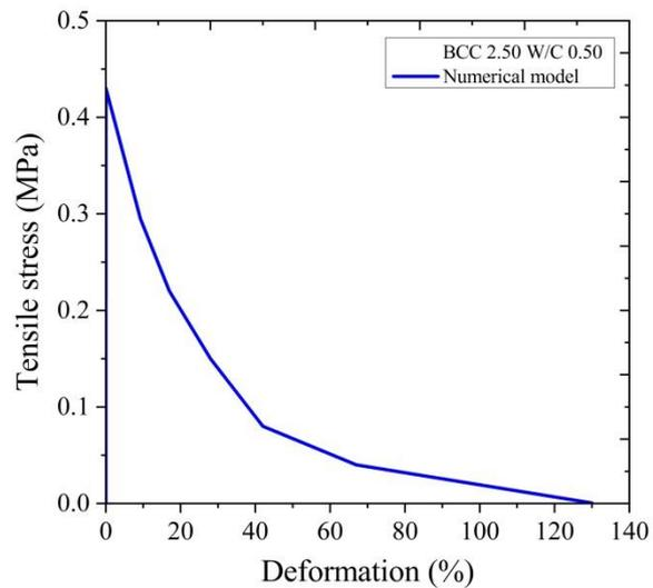
Figure 8. Graphical representation of the final tensile multilinear diagram BCC 2.50 W/C 0.50
