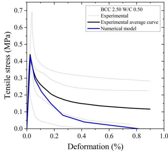
Figure 11. Tensile curves BCC 2.50 W/C 0.50
