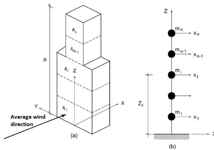
Figure 1. Discrete model. (modified from NBR 6123:2023 [1])
