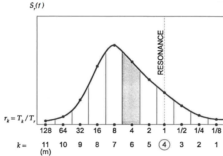
Figure 3. Reduced power spectrum decomposition into 11 parts (Franco [2]).
