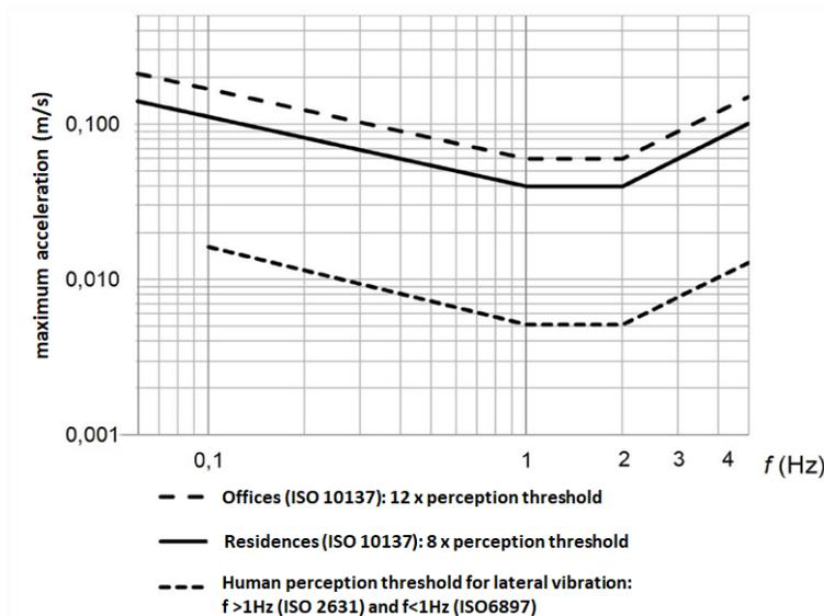
Figure 2. Human comfort. (modified from NBR 6123:2023 [1])
