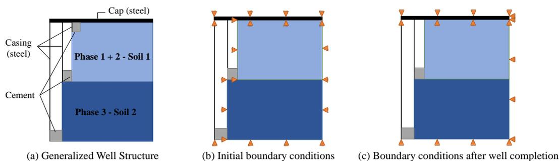
Figure 1. Study scenario with two annuli and material assignment for each region of the model
