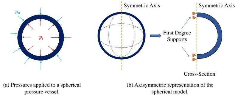
Figure 2. Representative model of a spherical pressure vessel
