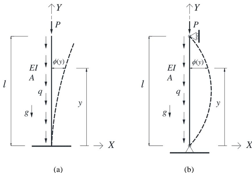
Figure 1. (a) clamped-free case ( $CF$ ), (b) hinged-hinged case ( $HH$ )
