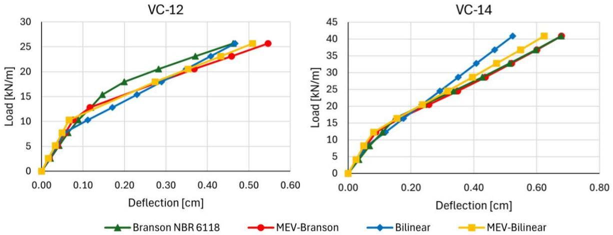
Figure 2 - Load-deflection graphs for beams VC-12 and VC-14
