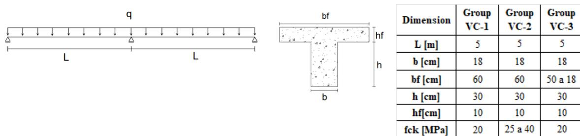
Figure 1- Loading type, beam dimensions, and geometry.
