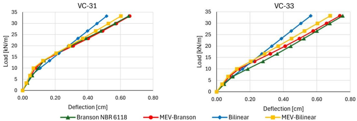
Figure 4- Load-deflection graphs for beams VC-31 and VC-33.
