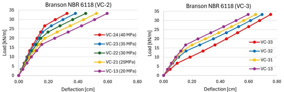
Figure 3- Load-deflection graph for Group 2 and Group 3 beams according to the Branson NBR 6118 method
