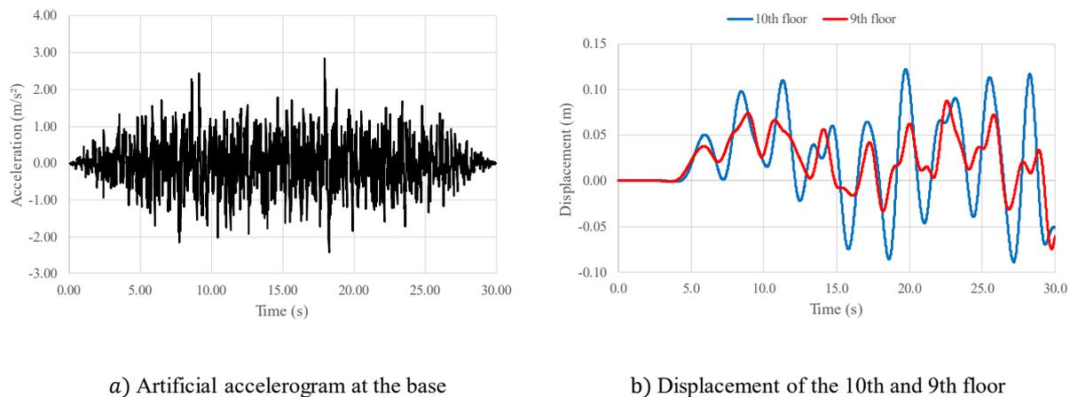
Figure 5. Artificial accelerogram and displacement of the 10th and 9th floor
