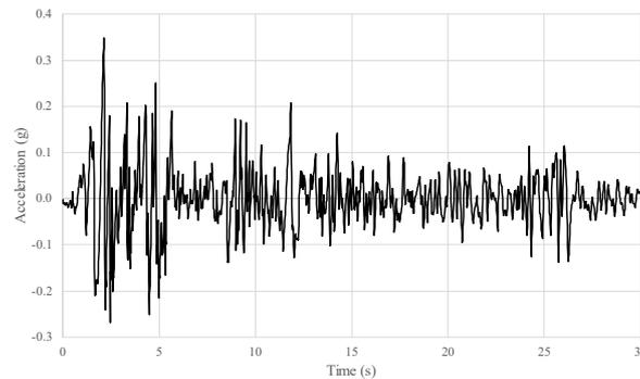
Figure 2. Accelerogram El Centro earthquake (N-S component)
