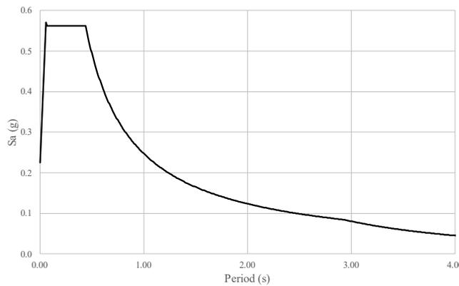
Figure 3. Target response spectrum.
