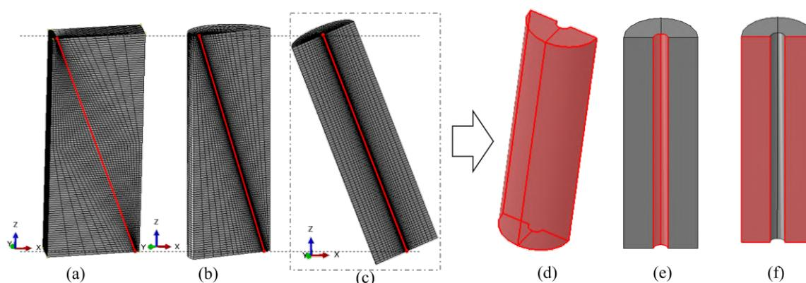
Figure 1. (a, b, c) Geometry attempts for modeling the massif; (d, e, f) Sets to define loads and boundary conditions.
