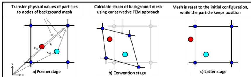
Figure 1 : Schematic figure of typical computational mesh and particles [4]
