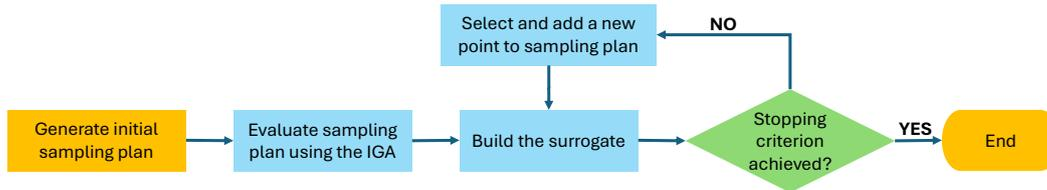
Figure 2. Flowchart of SAO using Kriging.
