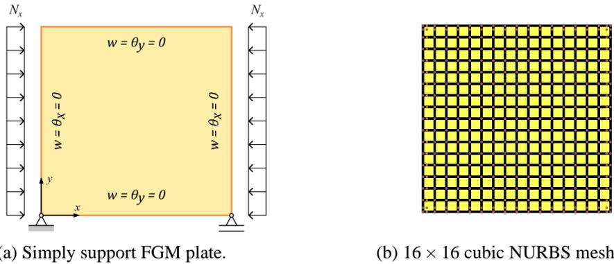
Figure 3. Simply support FGM plate and mesh used for the maximization of the buckling load.
