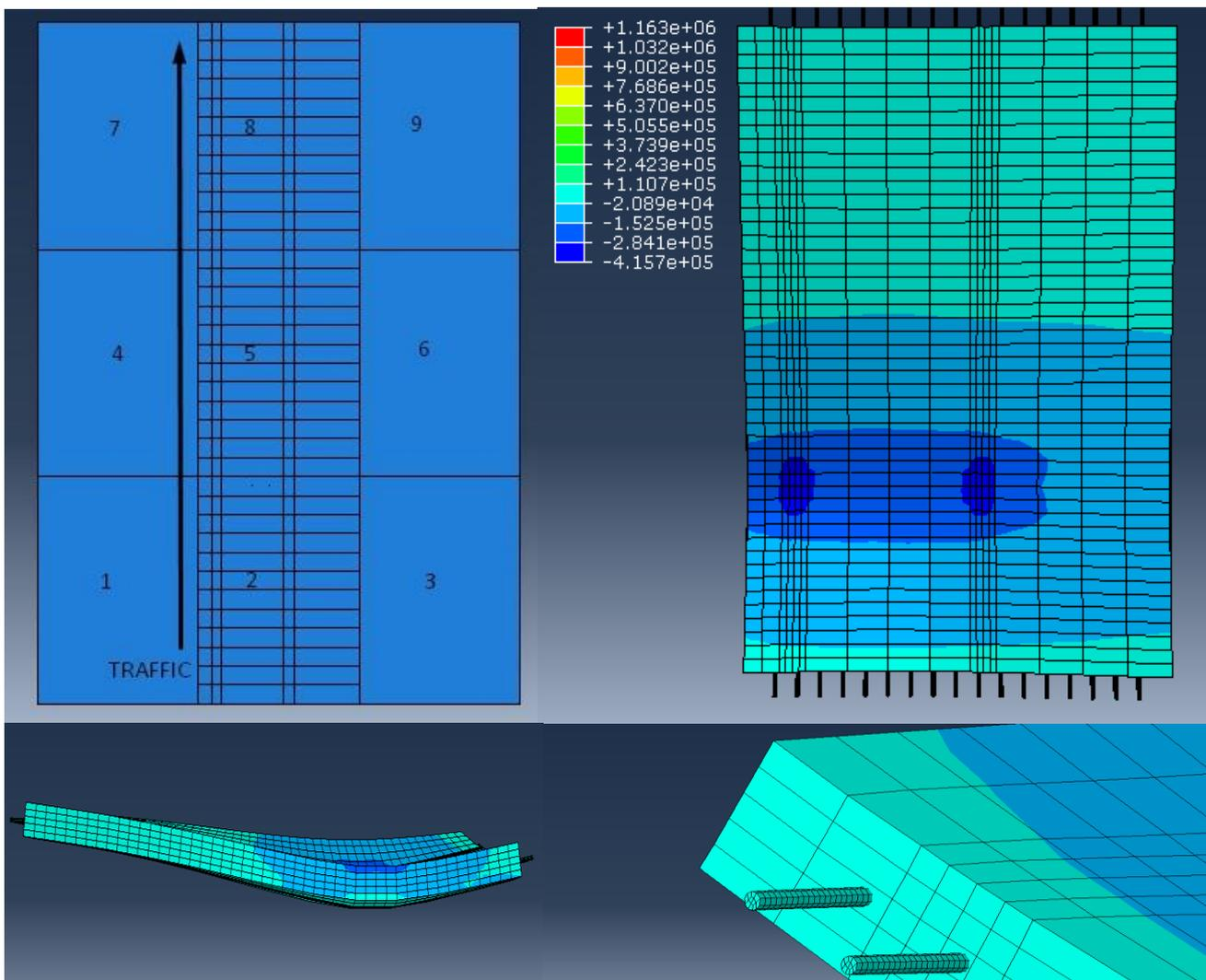
Figure 2. Example of a FEA Model. a) Assembly of the Model and Slabs numeration; b) Top view of deformed slab 5; c) Left view of deformed slab 5; d) Dowel Bar embedded into slab
