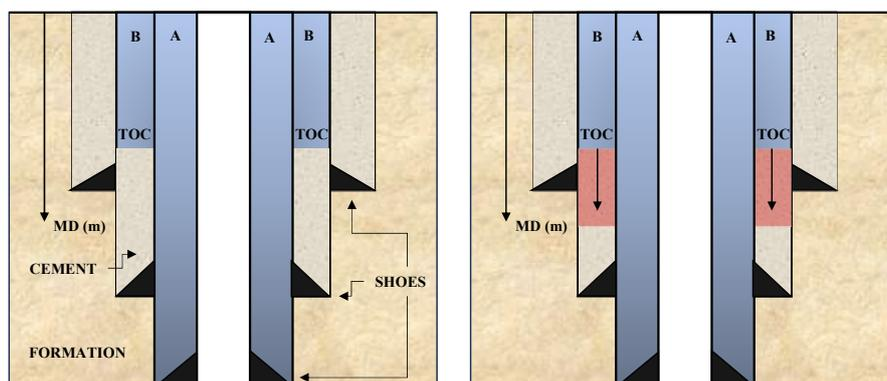
Figure 2. Representation of the reference well scenario with varying TOC heights
