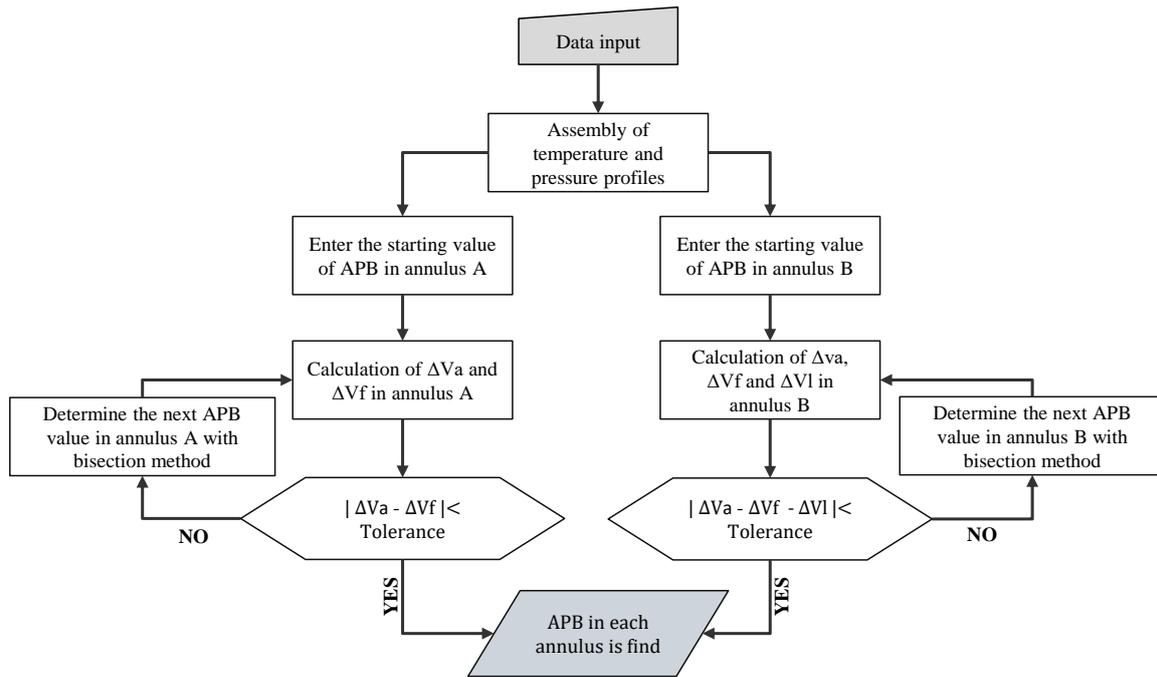
Figure 1. Flowchart for APB calculation (adapted from Wang et al. [4])
