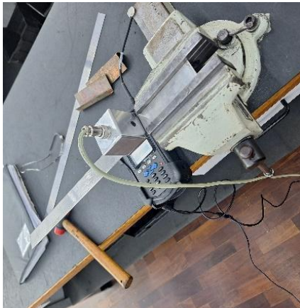
Figure 4. Validation of the clamped beam
