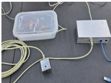
Figure 2 – Didactic acquisition system with the components arrangement.
