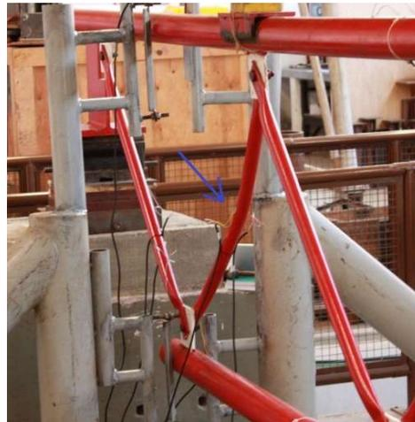
Figure 4. Buckling of the diagonal under compression (Mazon [20])
