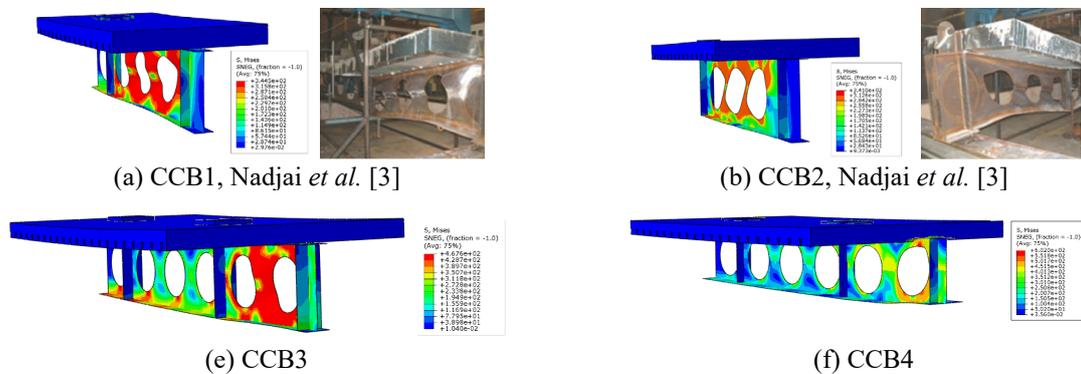
Figure 3: Deformed configuration of the validated beams
