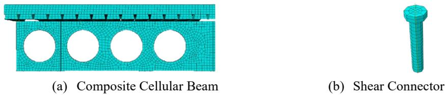
Figure 2: Discretization of elements
