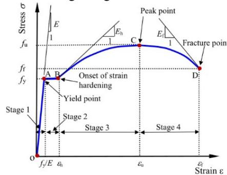
Figure 1: Discontinuous yielding model, Wang et al. [5]
