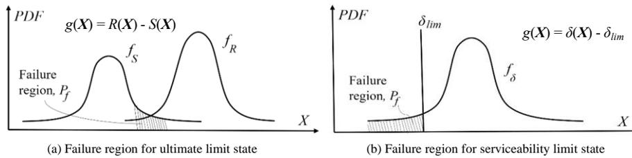
Figure 3. Failure region for different limit states.
