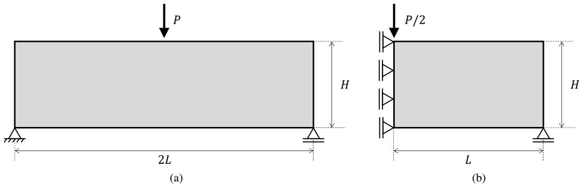
Figure 1. MBB beam problem, loading and support conditions: (a) full domain; (b) half of the domain considered due to problem symmetry.
