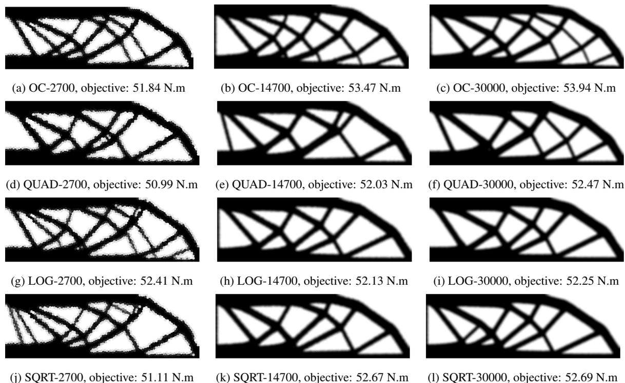
Figure 2. Final topologies for OC, CCSA-PSB quadratic (QUAD), CCSA-PSB logarithmic (LOG) and CCSA-PSB square root (SQRT) approximations, considering 2700, 14700 and 30000 elements.
