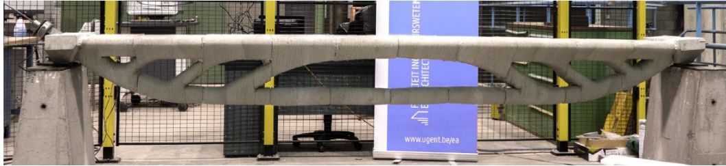
Figure 1. Concrete beam produced with the aid of 3D printing (Vantighem et al. [7])
