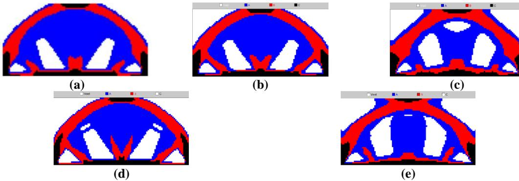
Figure 4 - Michell-type structure: (a) Zuo and Saitou [8]; (b) SIMP; (c) SESO; (d) SIMP with RBTO; (e) SESO with RBTO.
