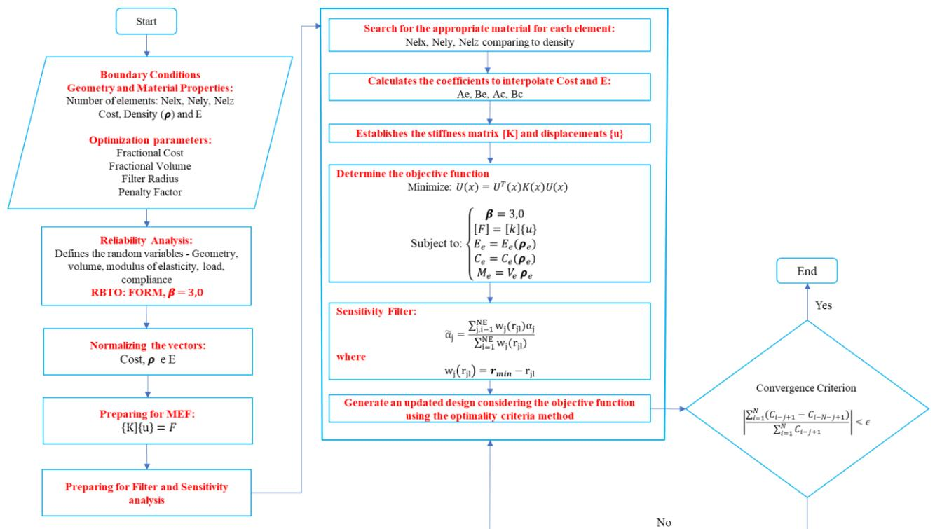
Figure 1 - Flowchart of the optimization process using the SIMP method
