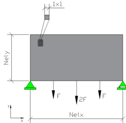
Figure 3 - Design of the Michell Structure with boundary conditions - 2D
