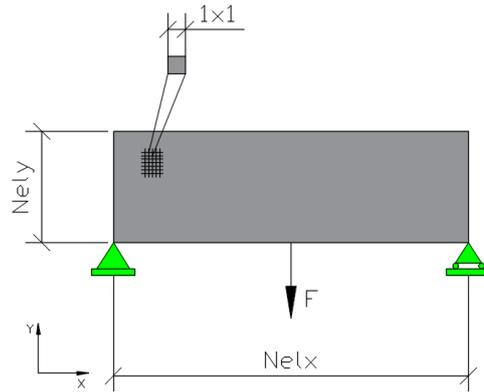
Figure 6 - Design of the MBB Beam Structure with boundary conditions - 2D
