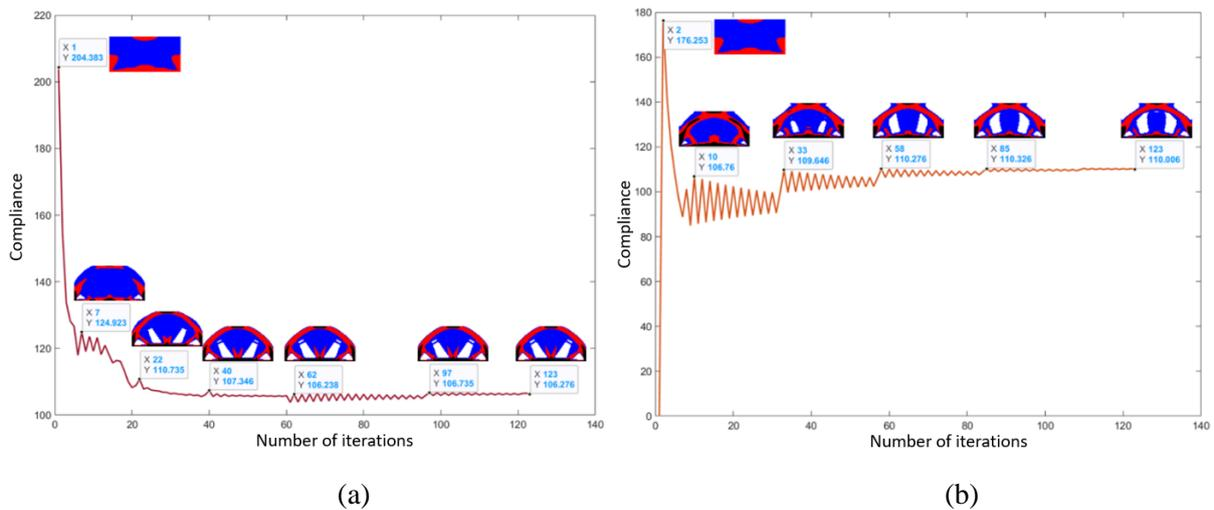
Figure 5 – Compliance by iteration number for Michell-type structure:
