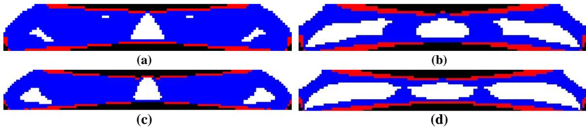
Figure 7 - MBB Beam Structure, MMTO: (a) SIMP; (b) SESO; (c) SIMP with RBTO; (d) SESO with RBTO.
