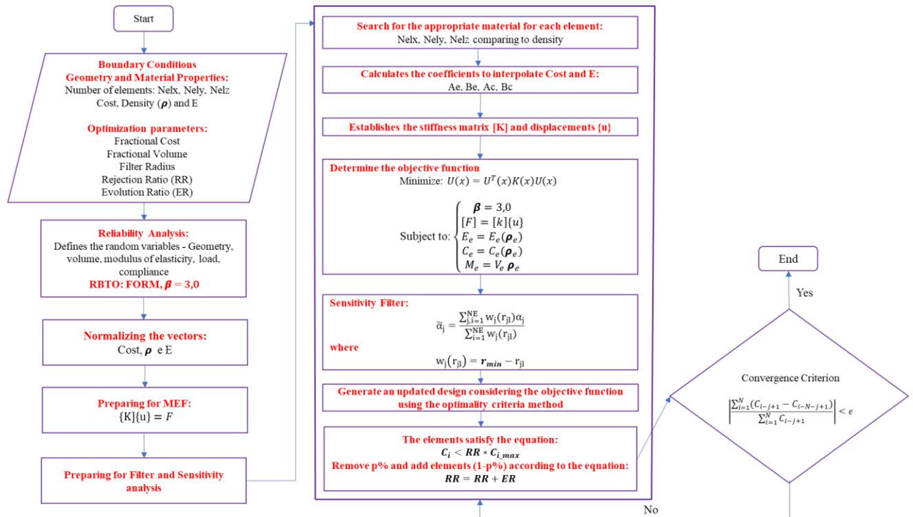
Figure 2 - Flowchart of the optimization process using the SESO method
