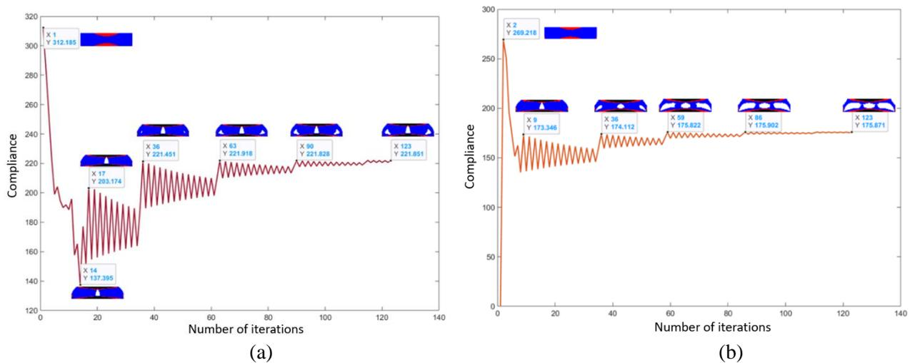
Figure 8 – Compliance by iteration number for MBB beam structure: (a) SIMP with RBTO; (b) SESO with RBTO.
