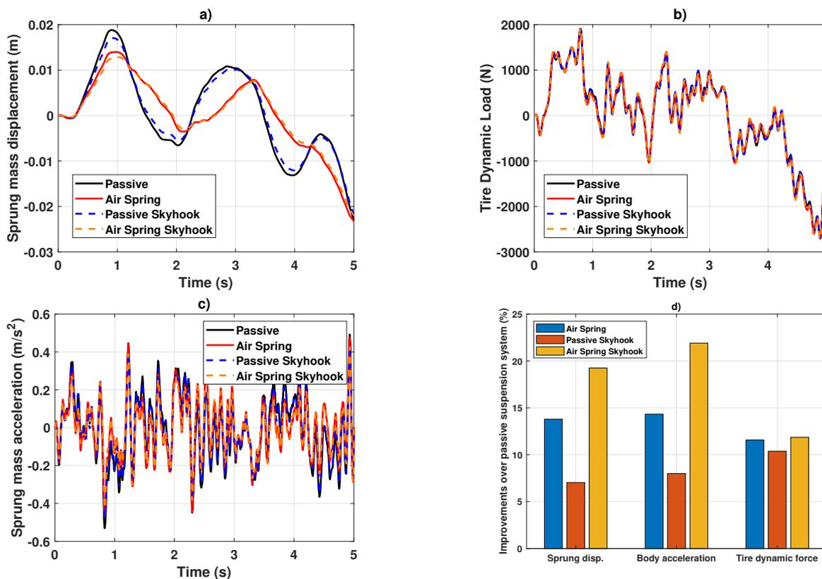
Figure 5. Dynamic results for random road excitation (Class C, 20 m/s) for passive and air-spring quarter-vehicle suspension with/without skyhook control. Figure (a) shows the sprung mass displacement, (b) the tire load signal, (c) the suspended mass accelerations, and (d) a comparison of improvements relative to passive suspension based on performance criteria eq. (14)-(16).
