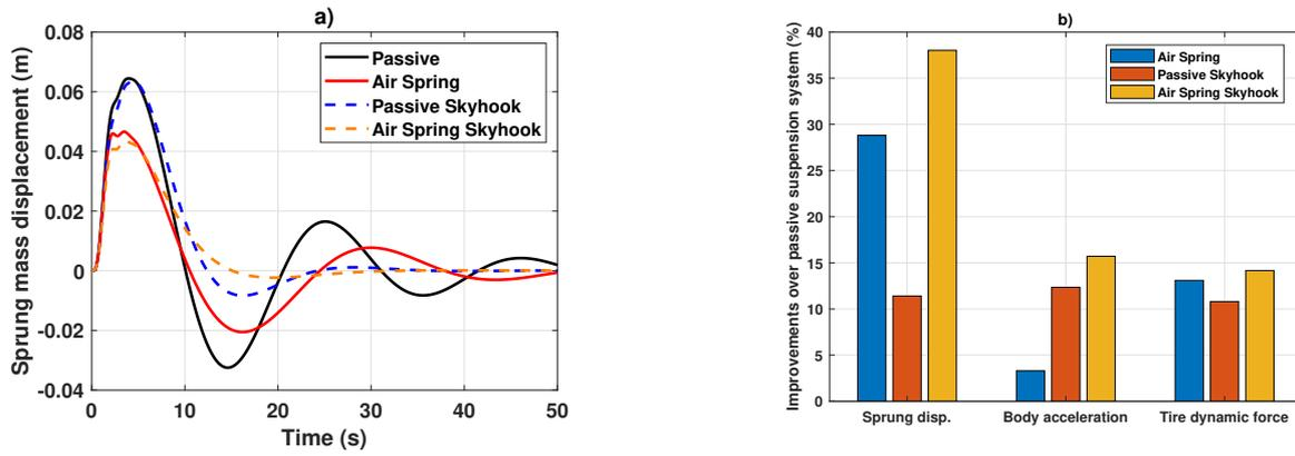
Figure 4. Dynamic results for sine wave excitation for passive and air-spring quarter-vehicle suspension with/without skyhook control. Figure (a) shows the sprung mass displacement, while (b) compares improvements relative to passive suspension based on performance criteria eq. (14)-(15).
