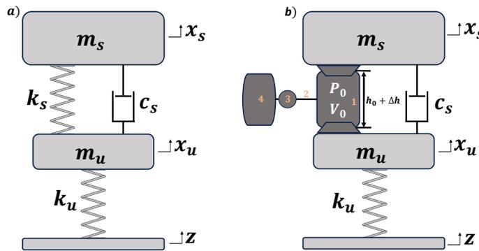
Figure 1. Schematic description of a quarter-vehicle system representation of (a) linear quarter of vehicle and (b) air spring quarter of vehicle. The index 1 in orange represents the air bag, 2 the connecting pipe, 3 the control valve (on/off), and 4 the reservoir.
