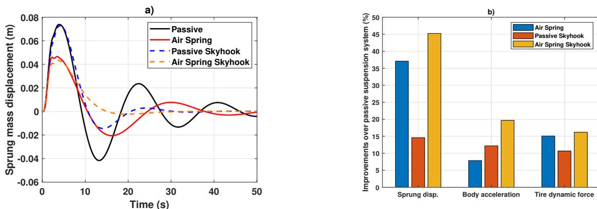
Figure 3. Dynamic results for bump excitation for passive and air-spring quarter vehicle suspension with/without skyhook semi-active control. Figure (a) shows time history of sprung mass displacement, while (b) shows comparison of improvement per report to passive quarter vehicle suspension as function of performance criterium eq. (14)-(15).
