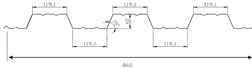
Figure 1. Typical deck-60 cross-section (dimensions in mm). Source: Costa [3]
