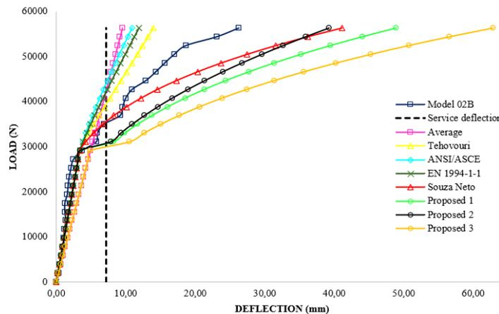
Figure 5 - Load versus deflection curve at mid-span considering creep of specimen 02B.
