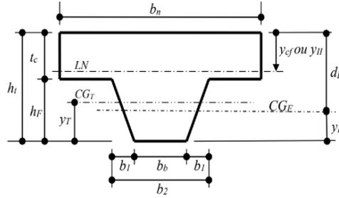
Figure 3: Typical cross-sectional modulus of the composite slab. Source: Costa [3].
