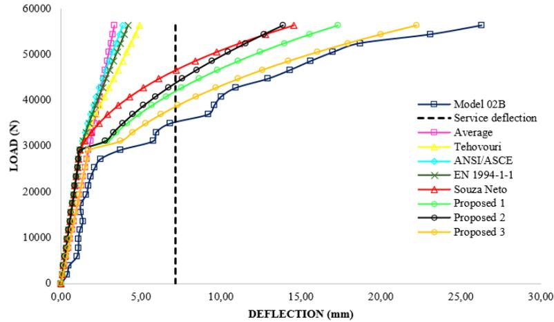
Figure 4: Load versus deflection curve at mid-span without considering creep of specimen 02B.
