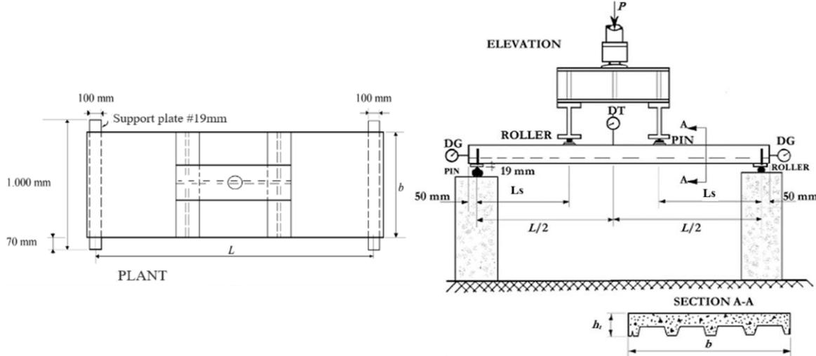
Figure 2 - Load application. Source: Costa [3]
