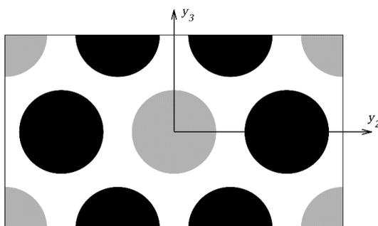
Figure 3. Repeating unit cell representative of the hybrid composite reinforced by two different types of continuous unidirectional fibers in a hexagonal array.
