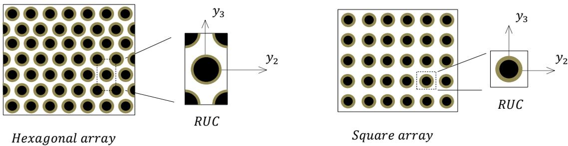
Fig. 2. Repeating unit cells for periodic composite reinforced by continuous fibers with interphase layers and different arrays.
