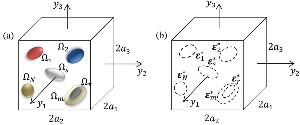
Figure 1. Generalized equivalent inclusion method; (a) Repeating unit cell with  $N$  inhomogeneities; (b) Homogenized unit cell embedding inclusions subjected to the eigenstrain fields.
