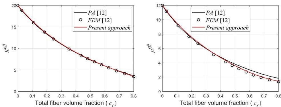
Figure 4. Effective elastic bulk and transverse shear moduli of the hybrid composite.
