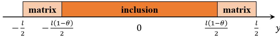
Figure 1. Periodic cell for matrix-inclusion-matrix case.
