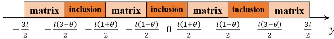
Figure 2. Periodic cell for matrix-inclusion-matrix-inclusion-matrix-inclusion-matrix case.
