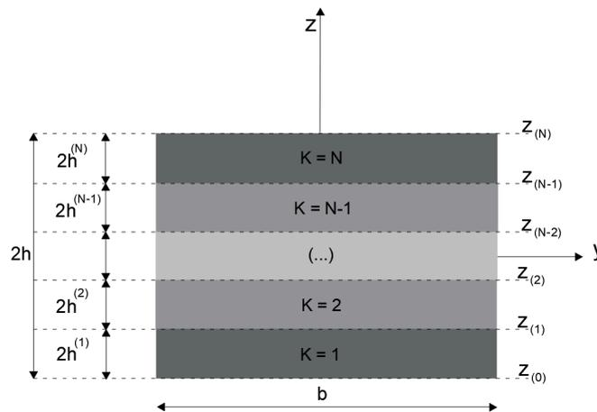
Figure 1. Section characteristics of a generic laminated beam.
