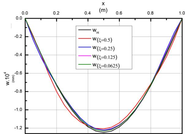
Figure 2. Convergence towards the homogenized solution  $w_H$  on maximum deflection of a beam with oscillating characteristics.
