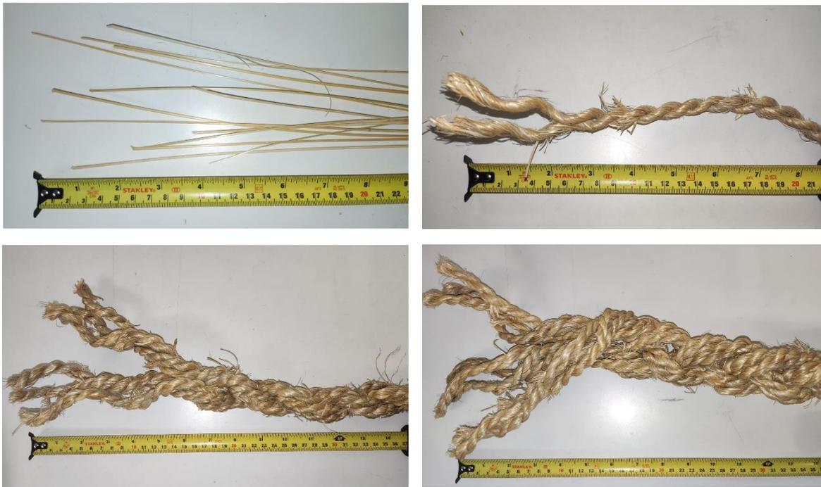
Figure 2. Q'oya fibers (upper left), Q'eswa type rope (upper right), Maqui type rope (lower left) and Duro type rope (lower right).
