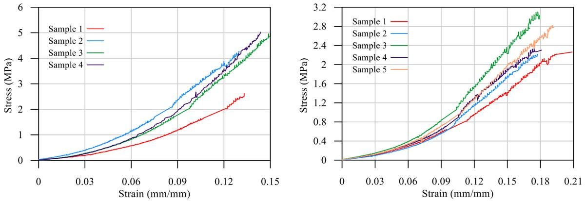
Figure 4. Tensile stress-strain curves of Maqui type (left) and Duro type (right) ropes.
