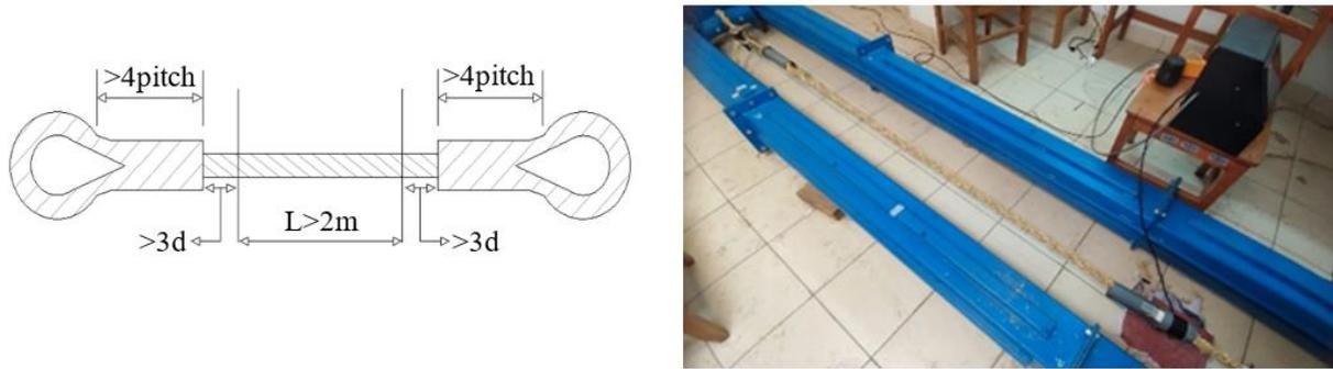
Figure 3. Minimum dimensions of a specimen (left) and tensile testing machine (right).
