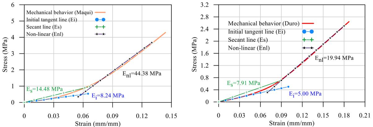
Figure 6. Modulus of elasticity of Maqui (left) and Duro (right) ropes.
