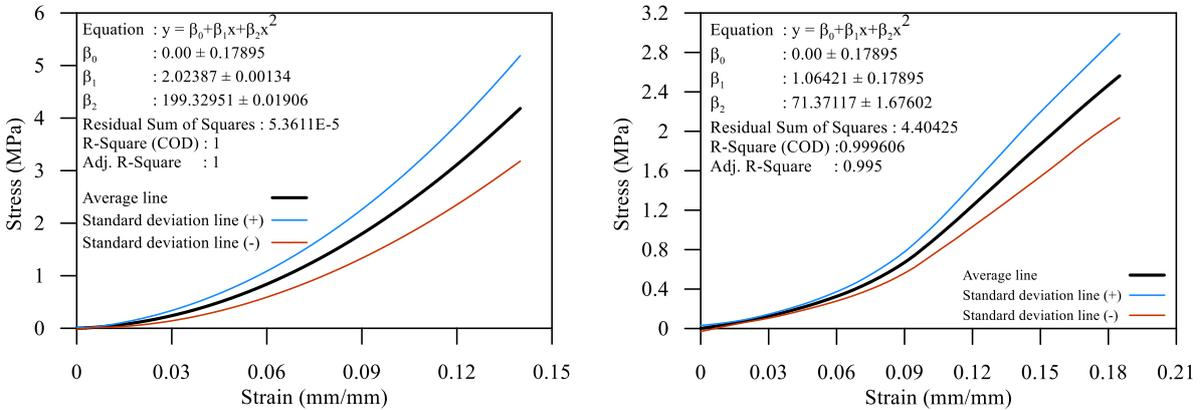
Figure 5. Stress-strain curves fitted with a polynomial approximation of Maqui (left) and Duro (right) ropes.
