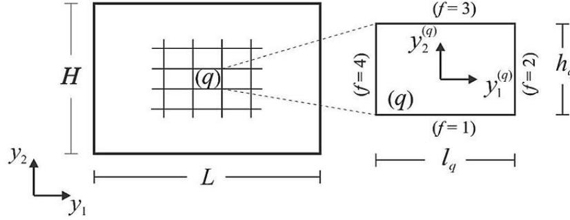
Figure 2. Discretized structure in rectangular subvolumes and local coordinate system of a generic subvolume  $q$ .
