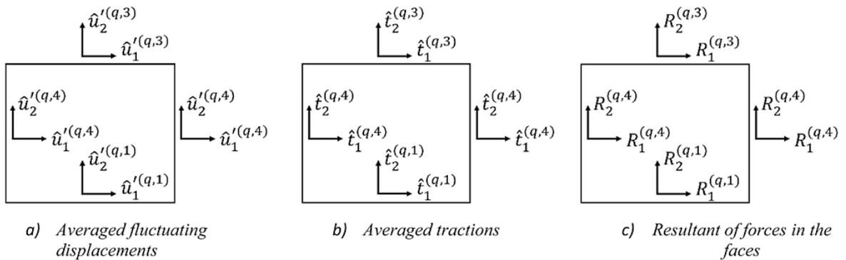
Figure 3. Surface kinematic and static quantities: (a) averaged fluctuating displacements; (b) averaged tractions; (c) resultant of forces in the faces.
