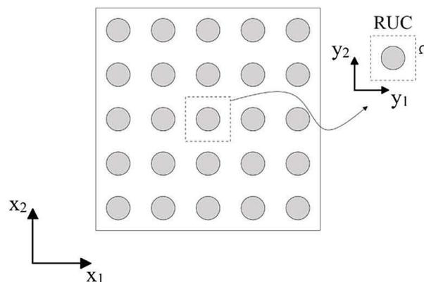
Figure 1. Periodic microstructure characterized by an RUC.
