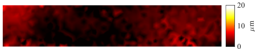
(b) Difference between the vertical displacement of the experimental measurement and finite element model values.
