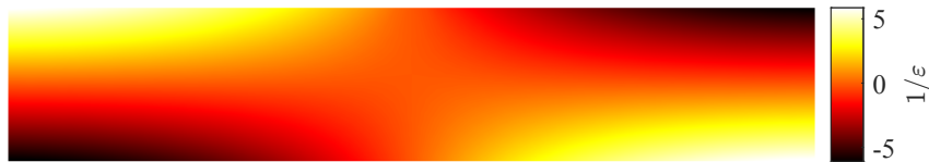
(a) Horizontal displacement sensitivity field, normalized by \gamma_U . Scale in 1/\epsilon , where \epsilon = 0.01 is the variation of E .
