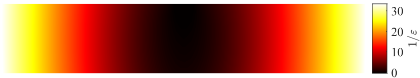
(b) Vertical displacement sensitivity field, normalized by \gamma_U . Scale in 1/\epsilon , where \epsilon = 0.01 is the variation of E .
