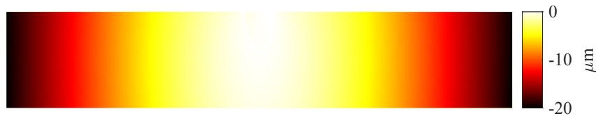
(a) Identified displacement field's vertical component.
