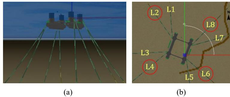
Figure 2. (a): Model of the studied platform; (b) top view of the model with numbered mooring lines. The lines chosen for the study are circled in red
