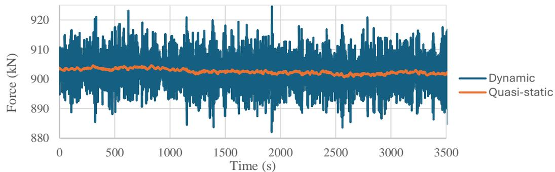
Figure 3. Graph of the tension series of a mooring line: Dynamic vs. Quasi-static
