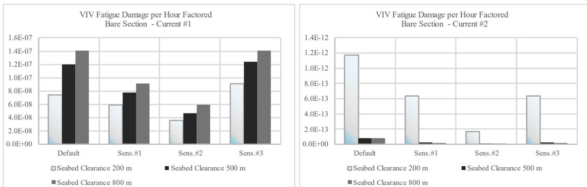
Figure 4. VIV Fatigue Damage per Hour Factored – Bare Section – Current #1 & Current #2
