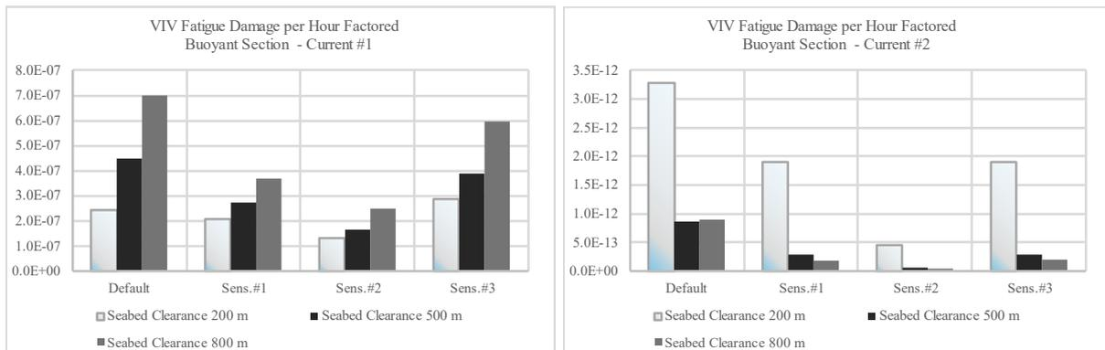
Figure 3. VIV Fatigue Damage per Hour Factored – Buoyant Section – Current #1 & Current #2
