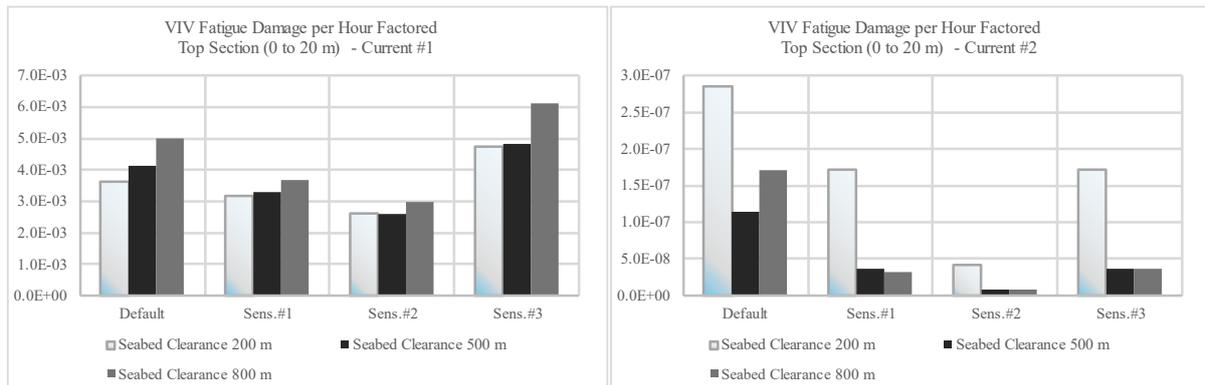
Figure 2. VIV Fatigue Damage per Hour Factored – Top Section (0 to 20m) – Current #1 & Current #2
