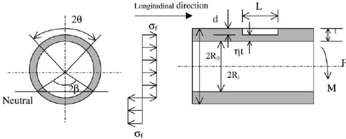
Figure 1. Pipeline geometry and corrosion defect, Zheng et al. [5]
