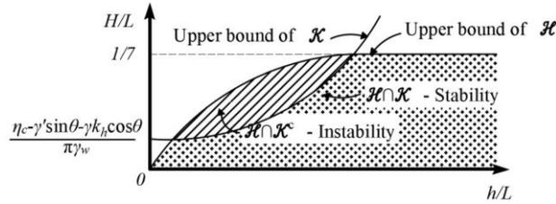
Figure 4. Boundary of the domain of safe loadings in the plane  $(H/L, h/L)$  in context pseudo-static
