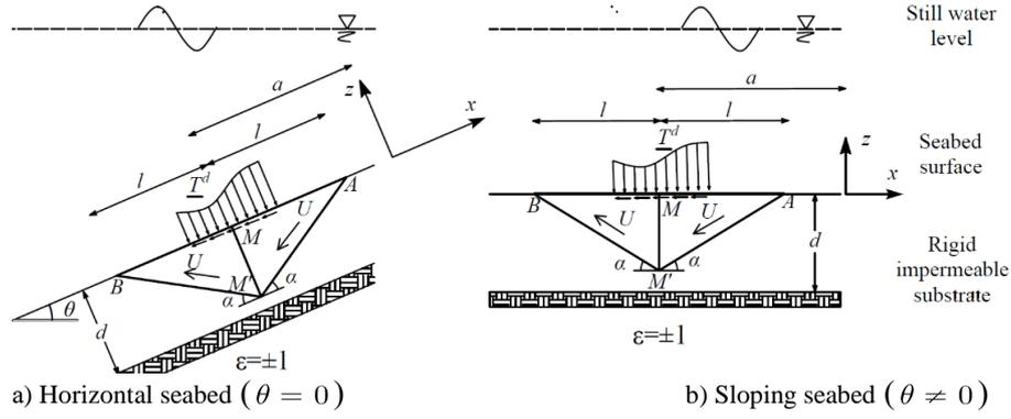
Figure 2. Piecewise rigid body motion velocity fields  $\underline{U}$
