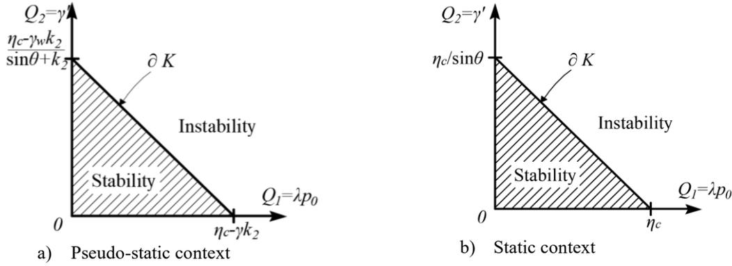
Figure 3. Domain  $K$  of supportable loading values  $(Q_1, Q_2)$  in the pseudo-static and static context
