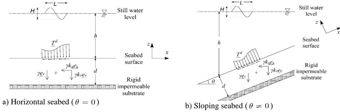
Figure 1. Geometry of the seabed subjected to wave loading and gravity force
