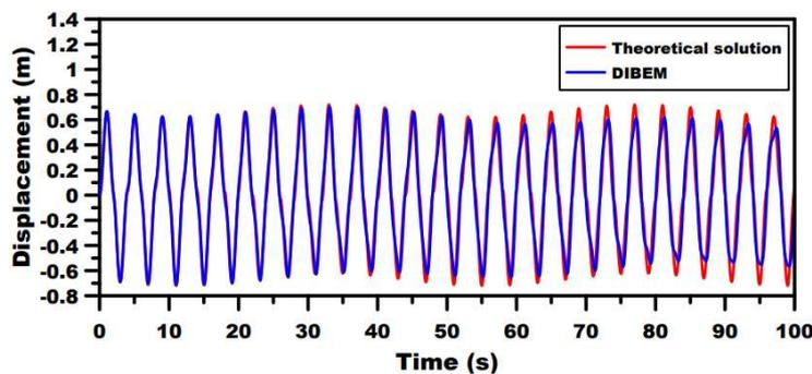
Figure 3. Displacement response with angular frequency of 3rd/s.
