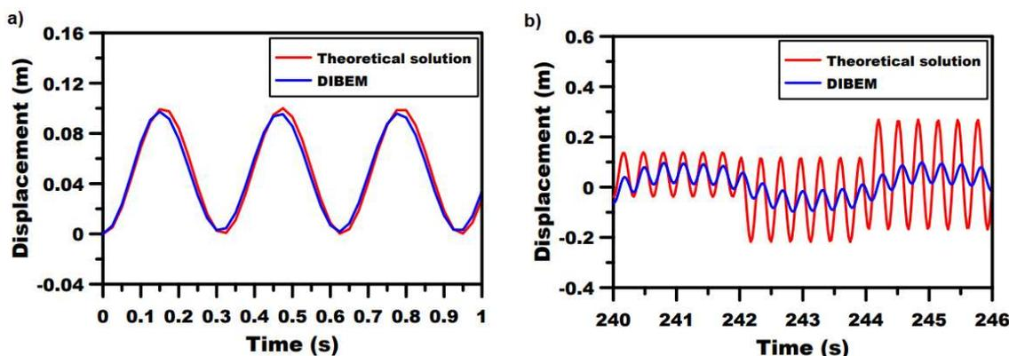
Figure 6. Displacement response with angular frequency of 20rd/s. (a) Starting times (b) Advanced times.
