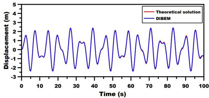
Figure 2. Displacement response with angular frequency of 1rd/s.
