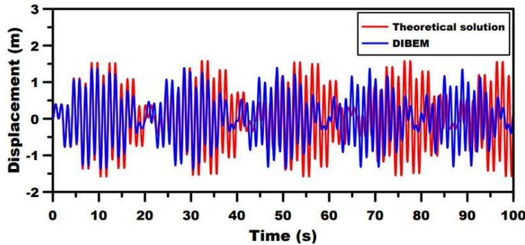
Figure 4. Displacement response with angular frequency of 5rd/s.
