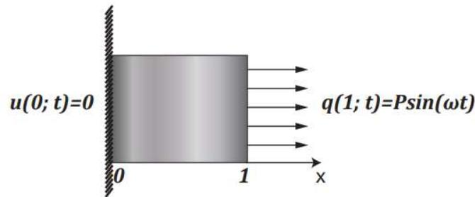
Figure 1. Bar subjected to time-varying load and boundary conditions.
