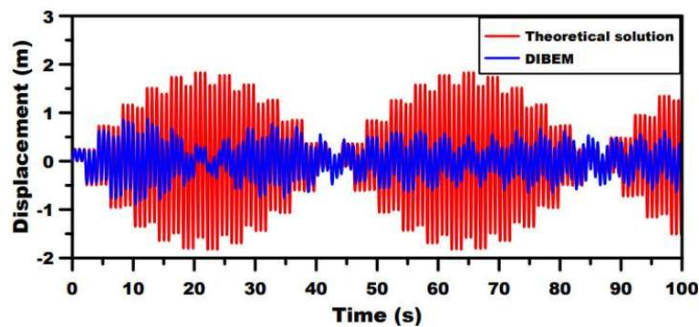
Figure 5. Displacement response with angular frequency of 8rd/s.
