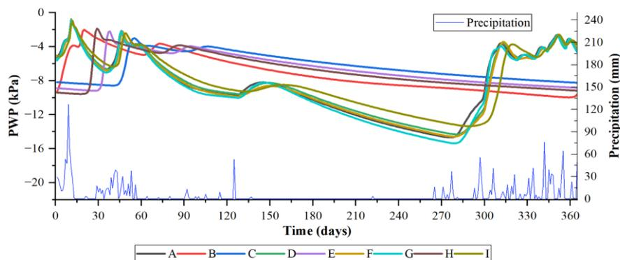
Figure 4. PWP in the embankment of the dam in scenario 2
