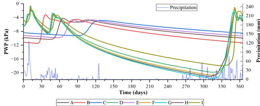
Figure 5. PWP in the embankment of the dam in scenario 3
